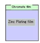
Thickness of chromate film: 0.2µm, Specific gravity: 5g/cm<sup>3</sup>
